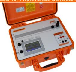
that the measured I-V-curves permit further explanations about the electrical characteristics of the verified module or string. That is why the PVPM 1540X is suitable as an instrument in research and for development purposes as well.
